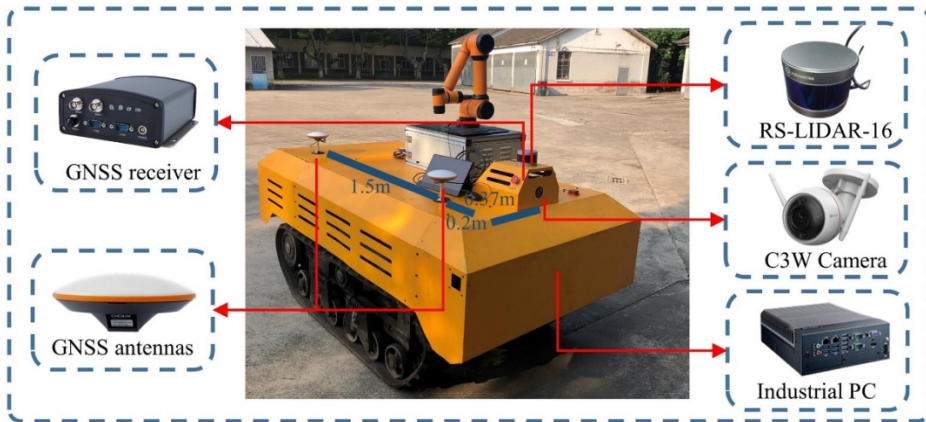
Figure 26. Research Robot Platform for VR Teleoperation (Wang et.al., 2024)
